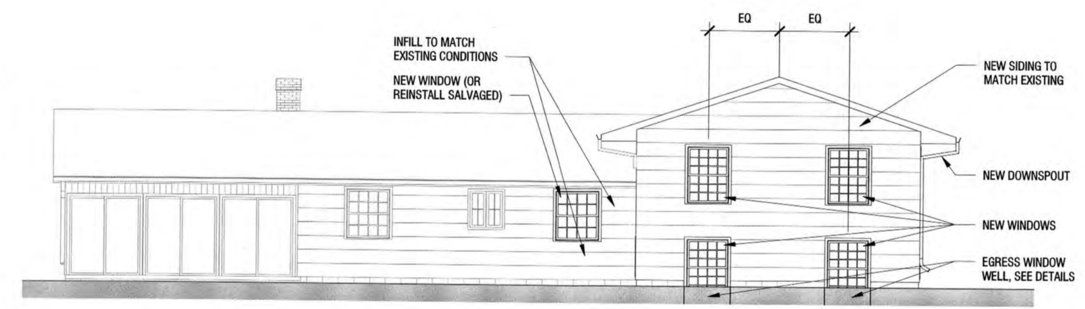
4 REAR ELEVATION - PROPOSED SCALE: 1/8" = 1'-0"
