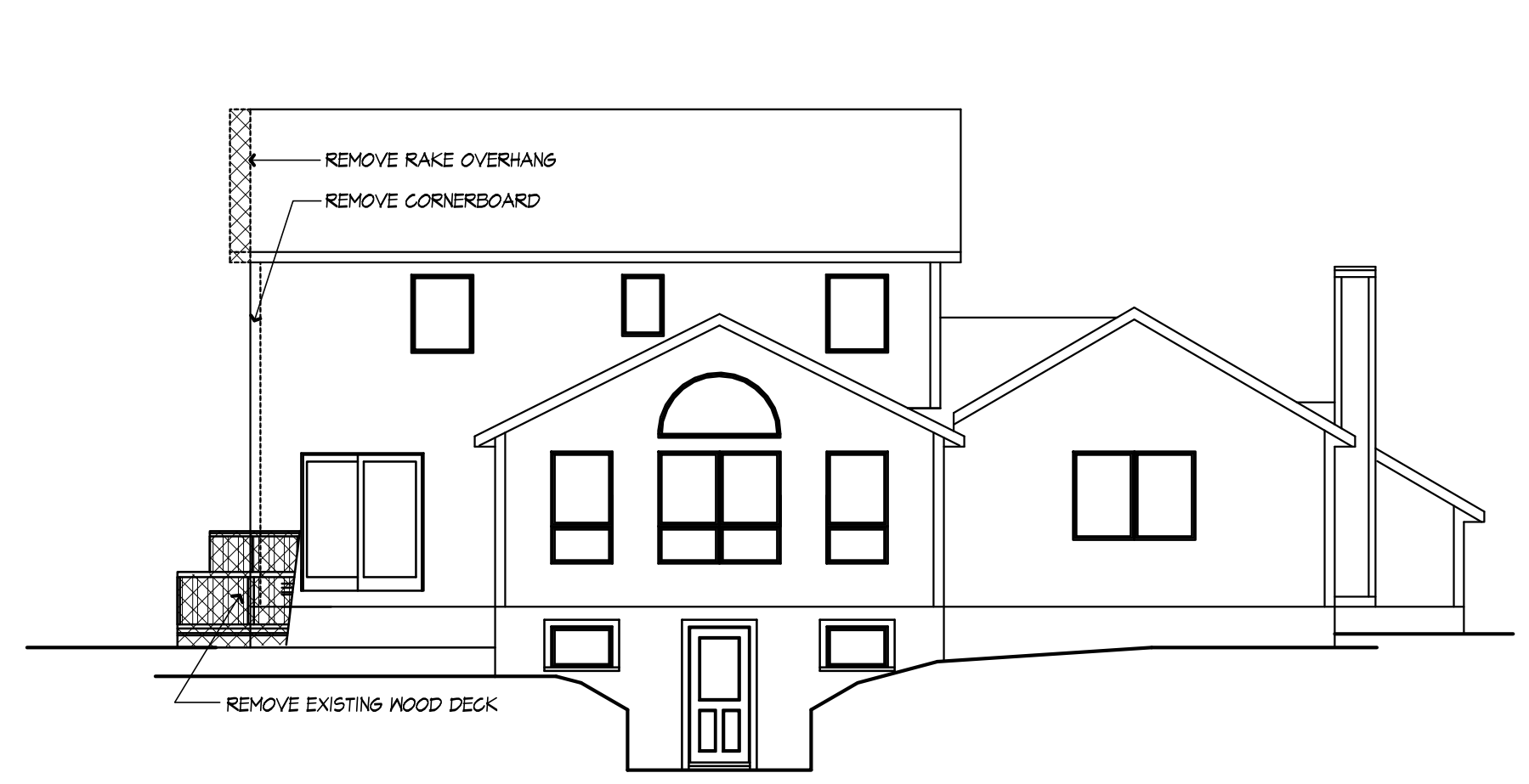
REAR ELEVATION / EXISTING WITH REMOVALS SHOWN SCALE: 1/8" = 1'-0"
