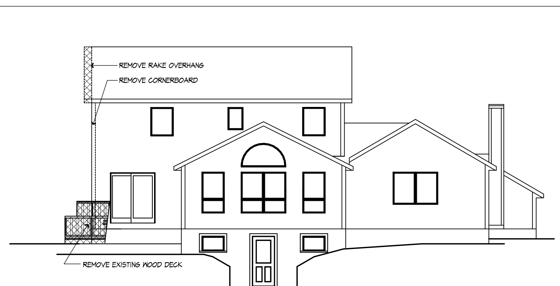
REAR ELEVATION / EXISTING WITH REMOVALS SHOWN SCALE: 1/8" = 1'-0"
