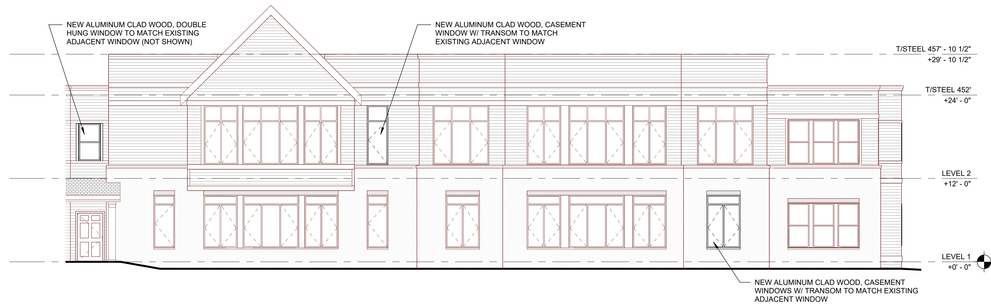
1B North Elevation - New Window Placement 1/8" = 1'-0"
