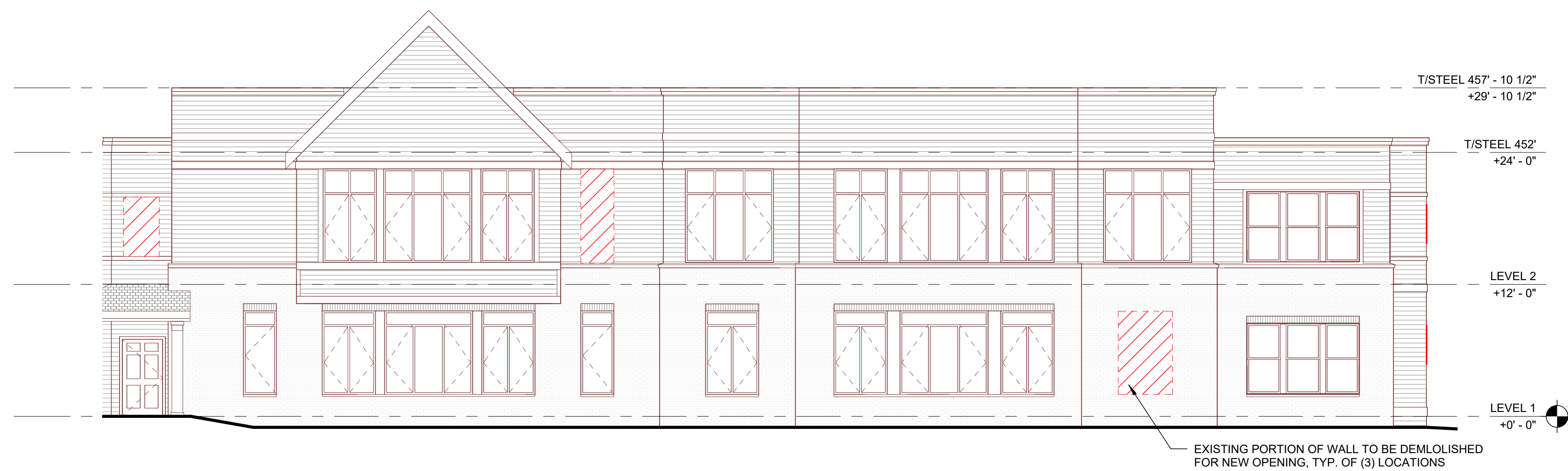
1A North Elevation - Existing 1/8" = 1'-0"
