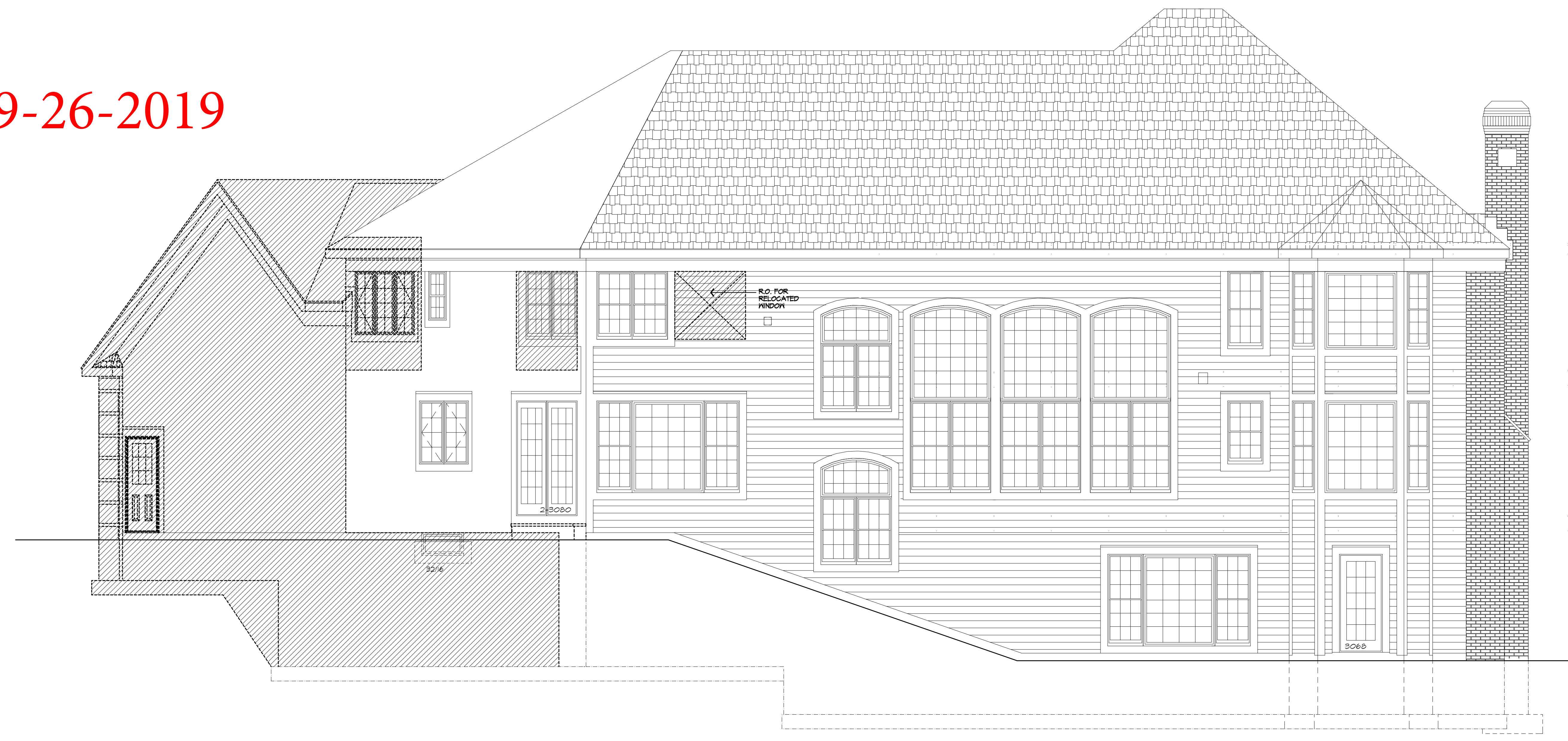
REAR ELEVATION/ EXISTING WITH REMOVALS SHOWN
