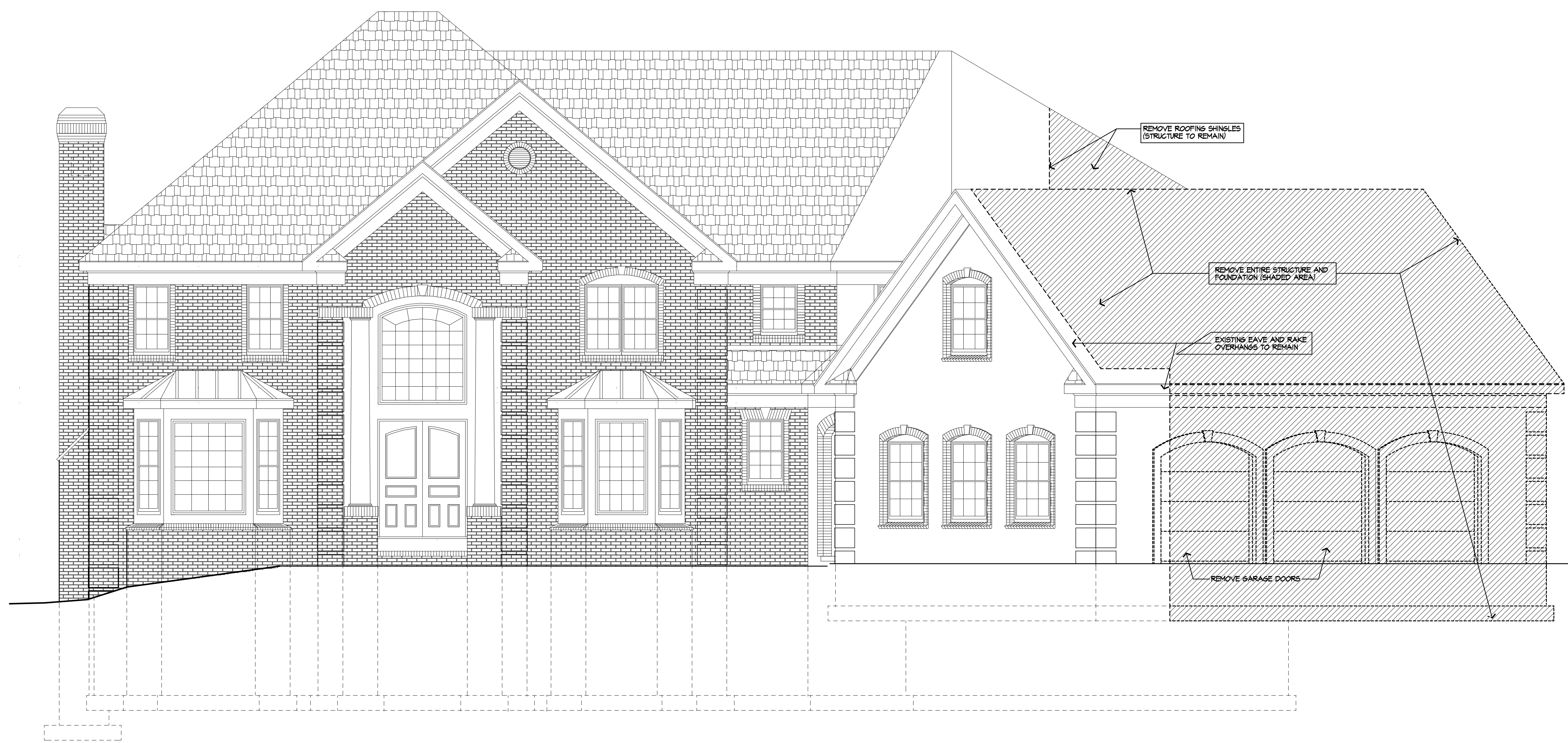
FRONT ELEVATION/ EXISTING WITH REMOVALS SHOWN
