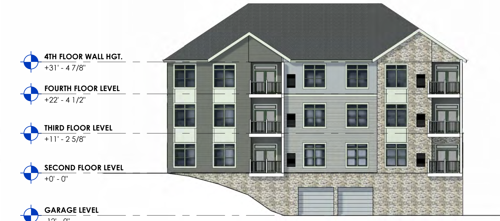
6 SOUTH ELEVATION EAST WING 0' 4' 8' 16' 32' 1/16" = 1'-0"
